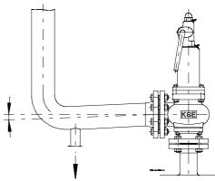
Lines for the drainage of condensate are to have adequate cross sections. They are to be laid with a gradient and must ensure safe drainage of the medium.
