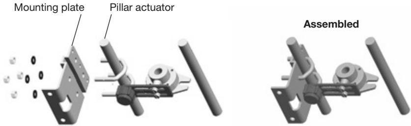
**Fig. 22** Pillar actuator assembly
