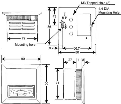
Fig.1 Dimensions in mm.-with baseplate and mounting plate model
