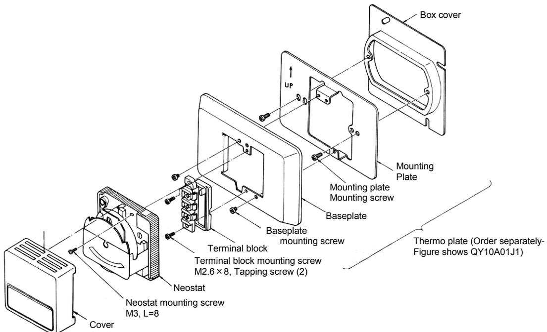
Fig.4 Mounting thermo plate
