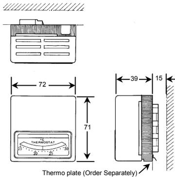
Fig.2 Dimensions in mm.-without baseplate and mounting plate model
