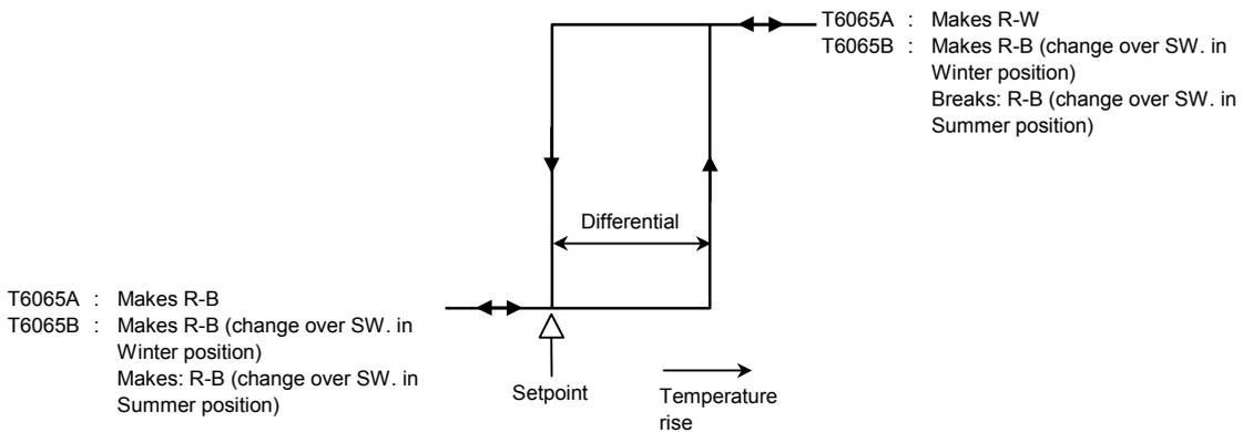
Fig.12 T6065A, B Switching action
