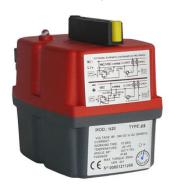
Protection against valve jams is provided by an electronic torque limiter, which autorelaxes the gearbox when activated, allowing the manual override to be selected to assist in clearing the jam. The effect of condensation is eliminated by an internal thermostatic anti-condensation heater that does not require a separate independent power supply.
