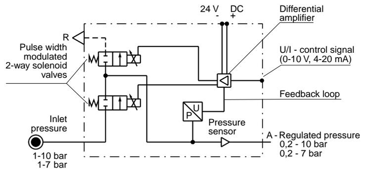
**3. EP-Transducer without pressure sensor and without output signal module.**
