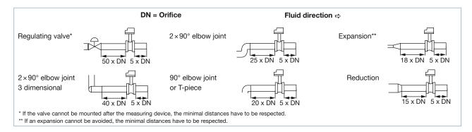
The device can be installed into either horizontal or vertical pipes. Important criteria for this are; ensure that the measurement pipe is fully filled and that the measurement pipe is air bubble free.
