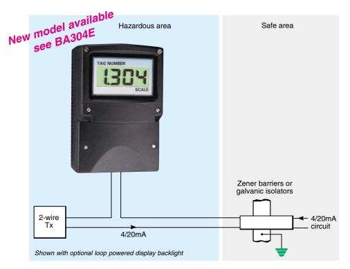
The new BA304D is a third generation intrinsically safe field mounting indicator housed in a robust IP66 GRP enclosure incorporating a separate terminal compartment and dedicated access to the instrument controls. Retaining all the features of the popular BA304C, this new indicator provides improved display visibility, plus simplified installation, calibration and routine inspection facilities.
