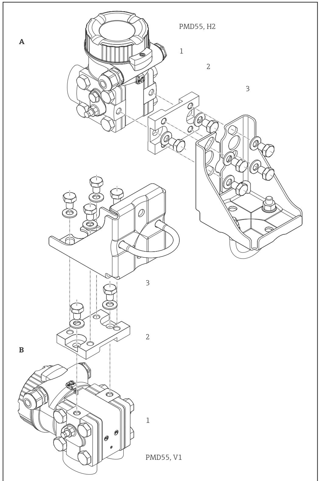
A Installation for horizontal impulse lines; H2 version
