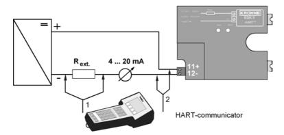
If a HART<sup>TM</sup> communicator (type Fisher Rosemount, Model 275) or a PC with HART<sup>TM</sup> modem is used, the resistor which is connected in series (Rext.) has to exceed 250 Ohms.
