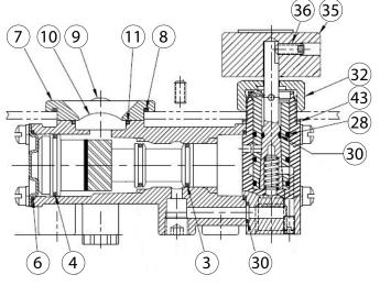
Indicating relay with TRIP port lockout and IN port bypass
